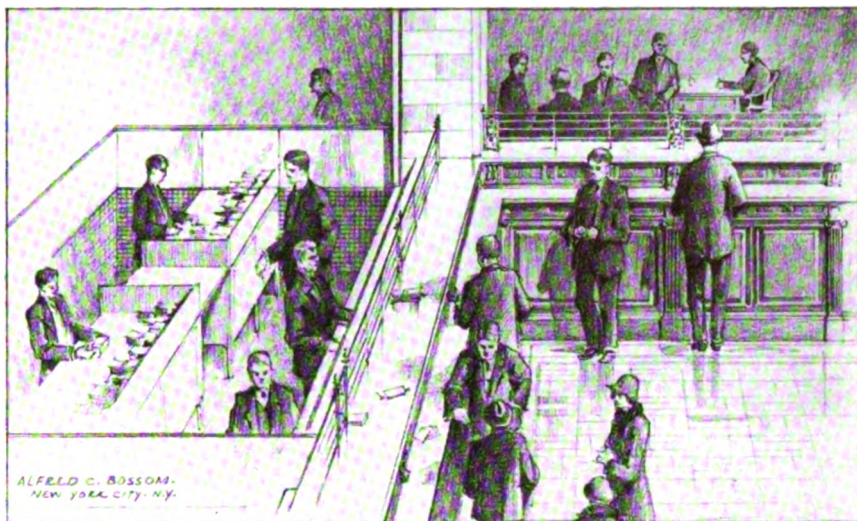
The new type of tellers' counter seen from above. Note how many more tellers can work in the same space behind the counter under this arrangement than with the usual barred wickets
