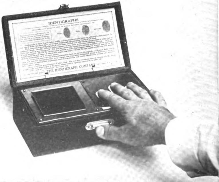
Put the card under shield and press the fingers in the three openings
