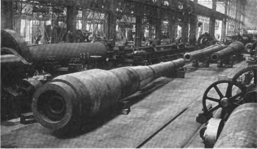
View of 16-inch Coast Defense Guns in process of manufacture, No. 2 gun shop, Bethlehem Steel Company
