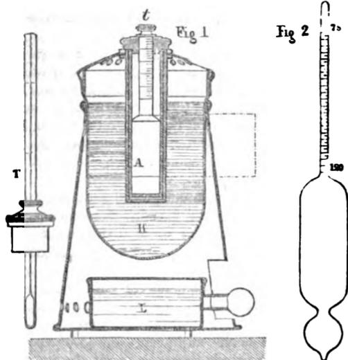
Fig. 1—M. Boland's "Aleurometre." *A*, closed cylinder, in copper. It is composed of two principal parts screwed together. *t*, copper tube, graduated into 25 spaces, from 25 to 50. *H*, oil bath. *T*, thermometer for ascertaining the temperature of the boiler.
